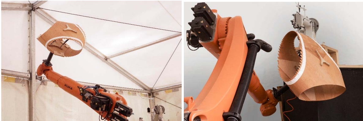
Robotic Sewing process of one segment. Three strips are held together by the robot's effector and lead through an industrial sewing machine to be permanently connected through stitches.
